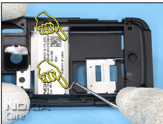
30. Unlock the two hooks of the C-COVER METAL PLATE.
