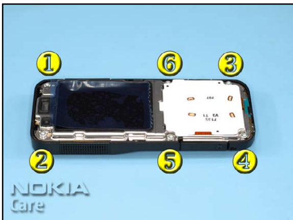
6. Tighten the six screws to the torque of 23Ncm in the order shown.
