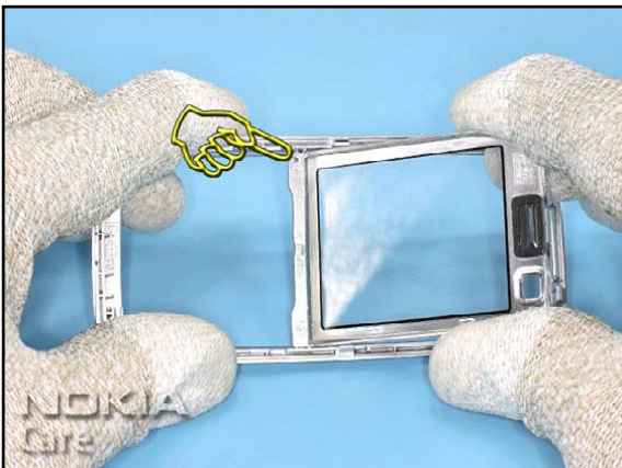
11. Pay attention to the guide pin of the WINDOW ASSY.
