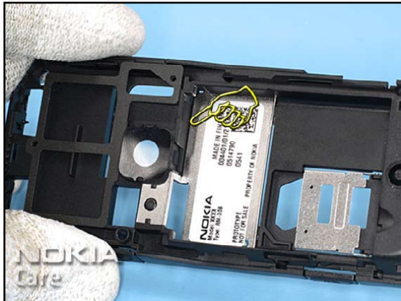
2. Place the C-COVER METAL PLATE onto the C-COVER as shown.
