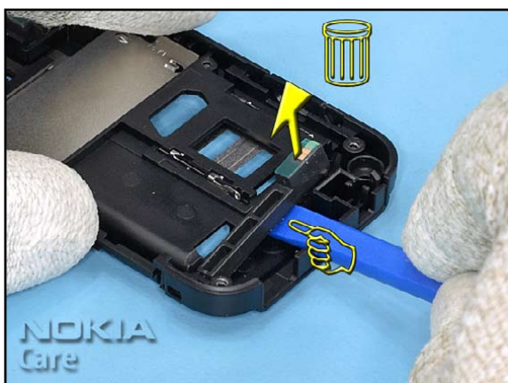
27. Lift the BT ASSY with the SS-93 as shown and discard it.
