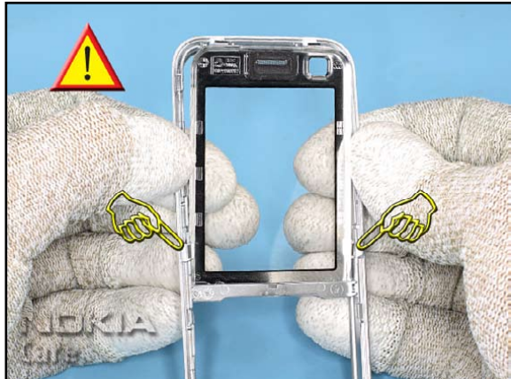
10. The WINDOW ASSY is additionally secured with two hooks to the A-COVER. Carefully expand the A-COVER a bit and then push out the WINDOW ASSY.
